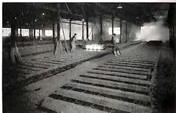
Here workers are pouring molten iron into molds to form top-quality cast iron soil pipe.
