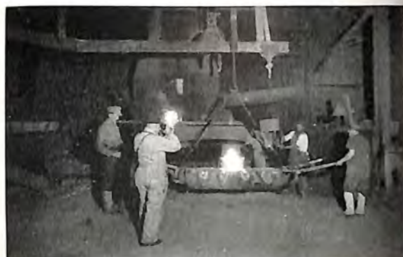
At the melting furnace, all metal poured is checked carefully for uniformity and correct mixture.
