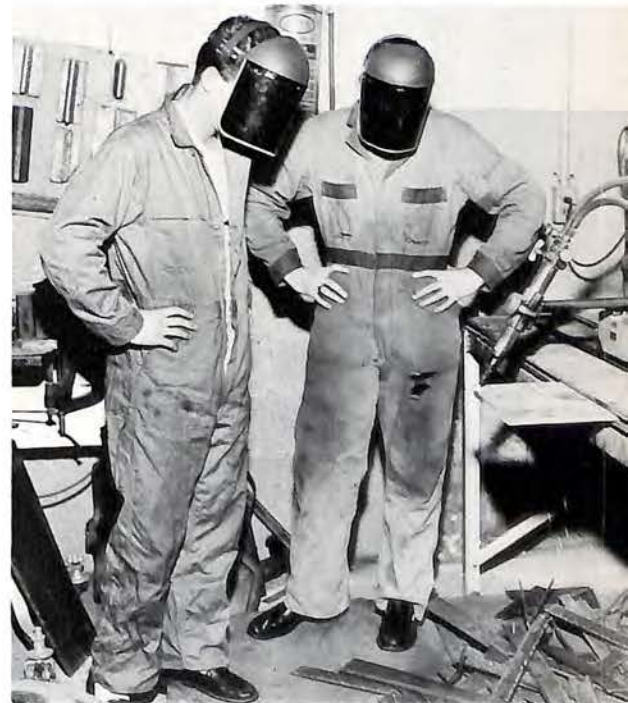
David Shank and Danny Bobbit cut 3/4 steel with automatic oxy-acetylene torch.
