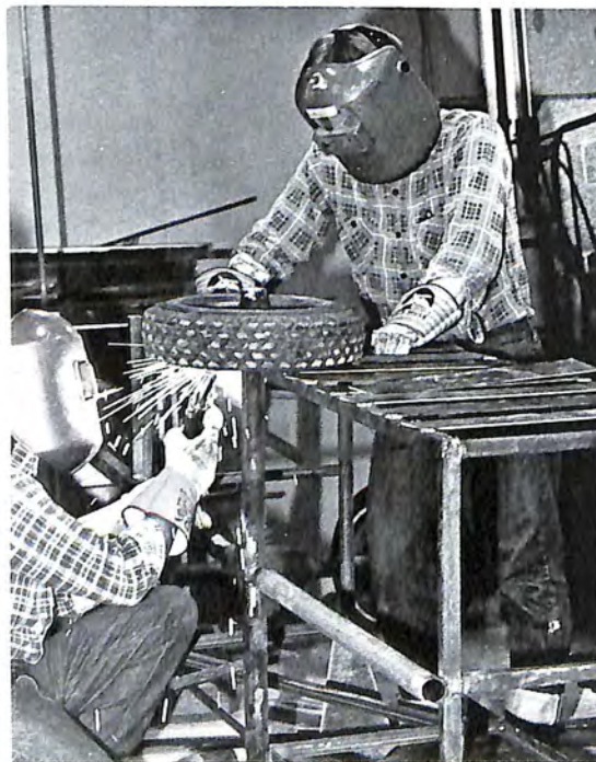
Sparks fly as Robert Beheler and Billy Batts weld an axle to the frame of a cart.
