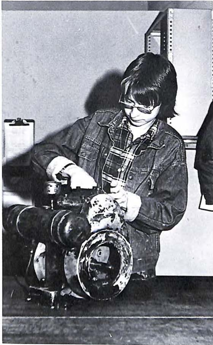
TINKERING Students taking the Small Engines class at RCEC rebuilt and repaired engines in motor cycles, go carts, and lawnmowers. Richard Clinebell changes the spark plugs in a 1930 model Briggs and Stratton engine.
