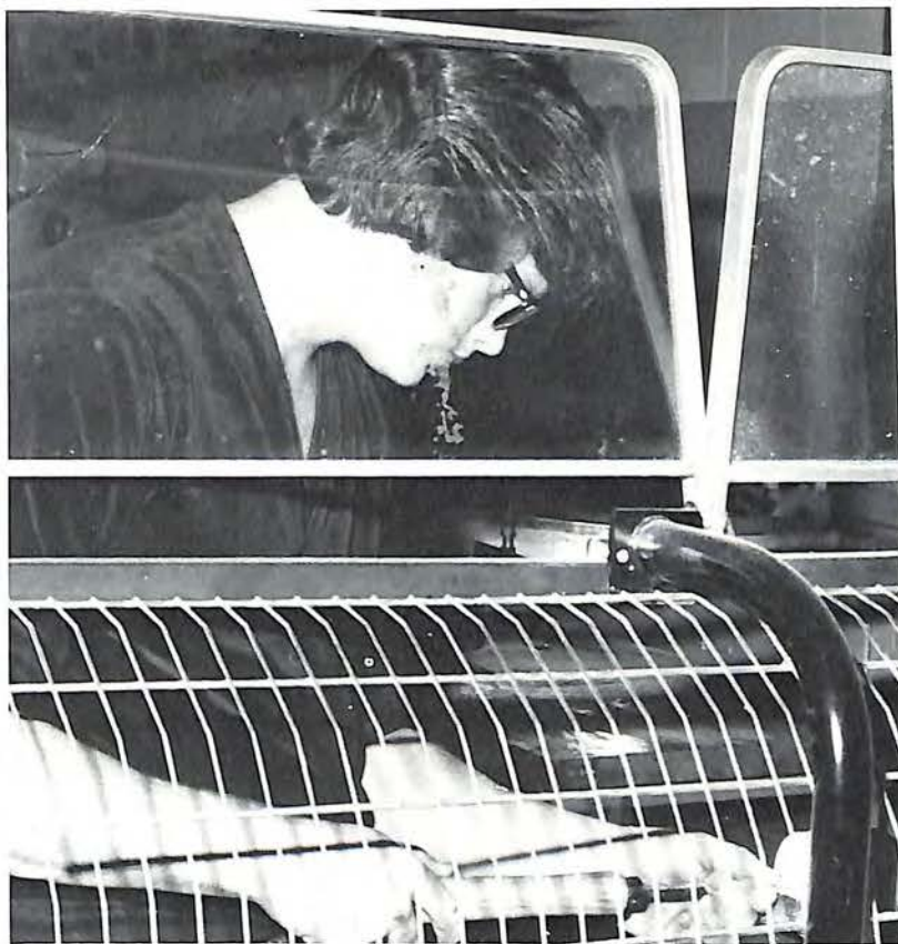
Steve Minnix turns a face plate on a wood lathe. The glass shield is a safety precaution, and part of the safety program which is followed assiduously.
