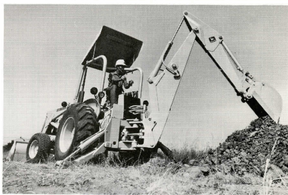
The detachable 9250-A Backhoe, with 2-lever control, digs 13 feet 8 inches and has a reach of 17 feet 5 inches.
