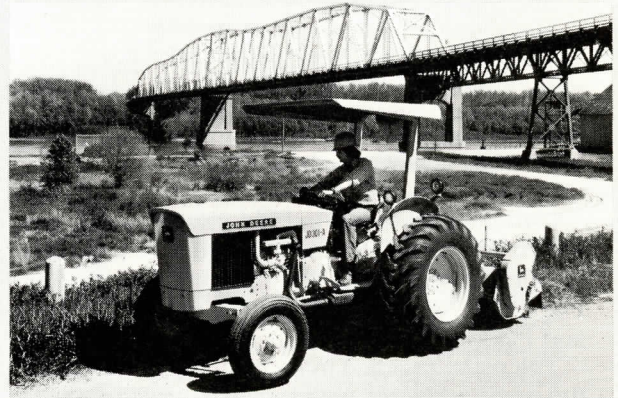
3-point lift links provide a vertical float action to follow ground contours, and adjustable sway blocks control side-to-side tool movement.
