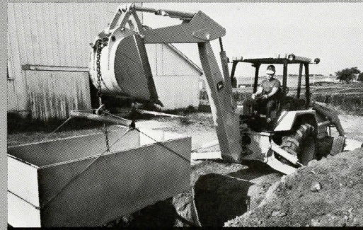
Low restriction, closed-center hydraulics provide powerful breakout and crowd forces, high lift and craning ability. Optional extendable dipperstick increases digging depth.
