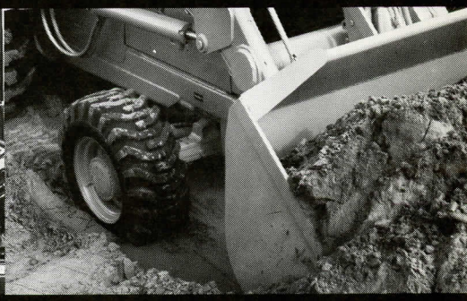
Optional mechanical front-wheel drive (scheduled for later availability) engages on the go, under load. Disengages automatically. Features a limited-slip differential.
