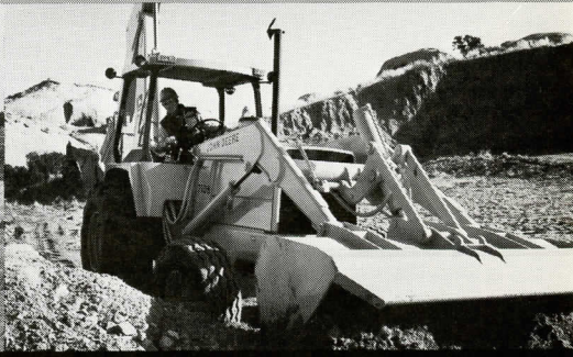
Boom arms that taper out to the bucket and a low boom knee height contribute to excellent visibility. A simplified linkage design also improves visibility, reduces weight, cuts maintenance.
