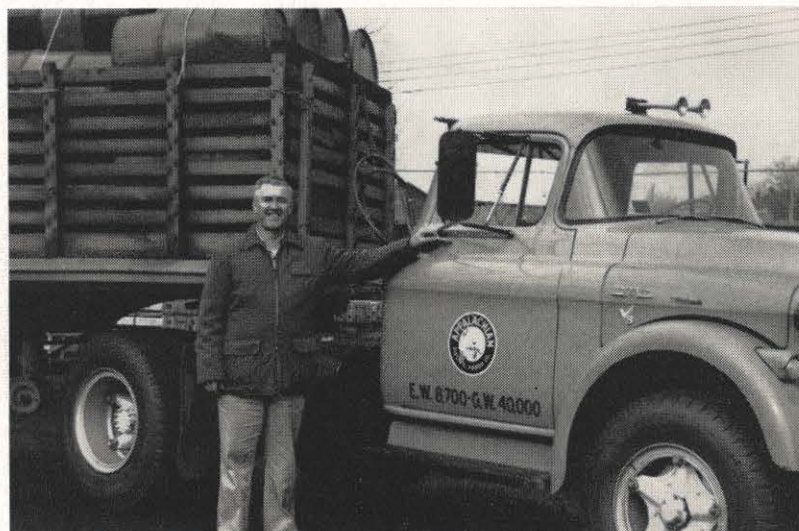
George E. Poole prepares to leave Roanoke on one of the many jobs he and his truck performs each year. The 90 empty 55-gallon oil drums on the truck were taken to the Ridgeway railway siding in the Fieldale district, where they were filled with oil from a transformer. The transformer had to be emptied to be within highway weight requirements when it was taken to the Ridgeway substation.
