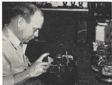
Repairing meters is another important part of work in the meter department. Here W. M. Mills, meterman, repairs a recording type demand meter.
