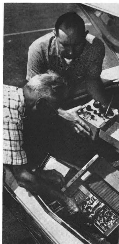
Adjustments and checking tests are made to a mobile radio unit in the trunk of a company car on the Roanoke office parking lot by E. E. Echols and G. W. Chilman.
