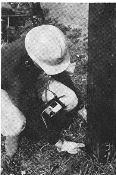
Soundness is checked with sound in a pole testing program Appalachian is trying out. Frequency of sound waves denotes the condition of the pole at the ground line.
