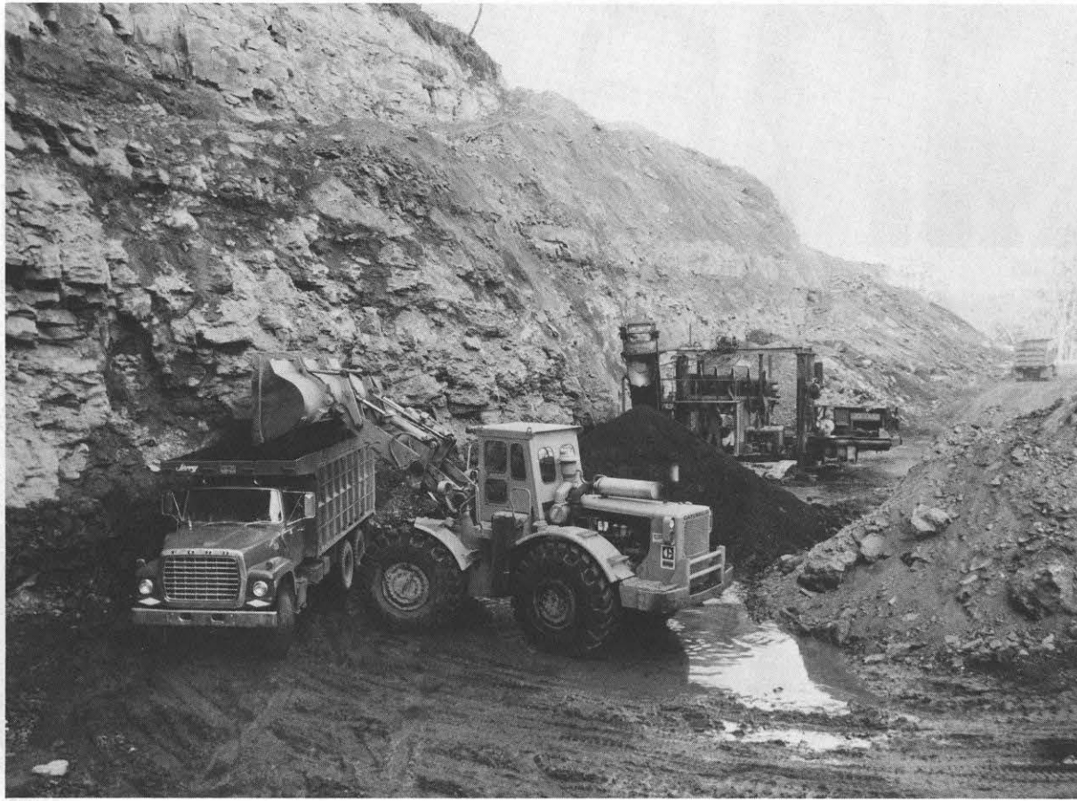
In contour mining, a "terrace" is cut into the side of a hill or mountain to expose the coal seam. Above are shown two methods of extracting the coal: digging the exposed coal (foreground) and auger-mining horizontally into the still-covered seam to remove still more coal (background).
