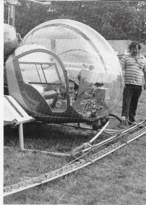
Appalachian was instrumental in the development of the .060 nozzle for use on the microfoil boom, as shown in this close-up photo of a helicopter used for spraying.
