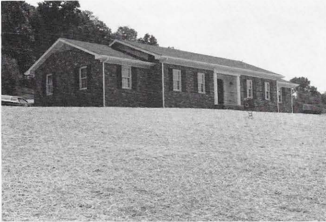
Kingsport Power Company's test home features a three-piece, high efficiency heat pump. The home's 52-gallon water heater is equipped with a "hot shot" which pre-warms the water, using waste heat from the heat pump.
